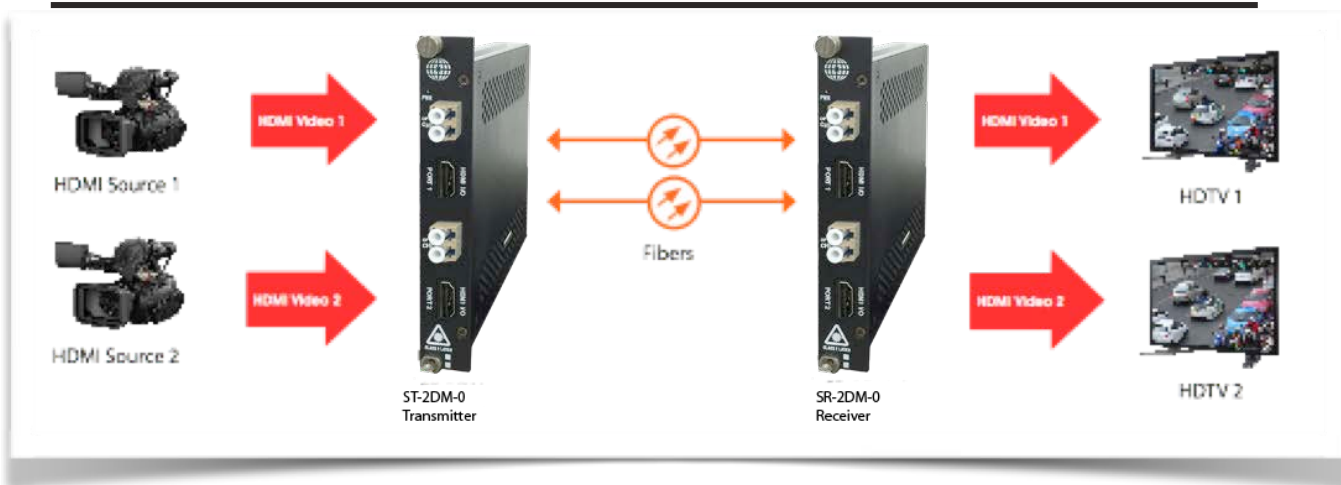
Figure 2. HDMI Optical Transceivers Connection (ST/SR-2DM-0 link shown)
