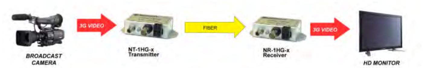
Figure 4.2 NT/NR-1HD(HG)-x Module Connection Diagram
