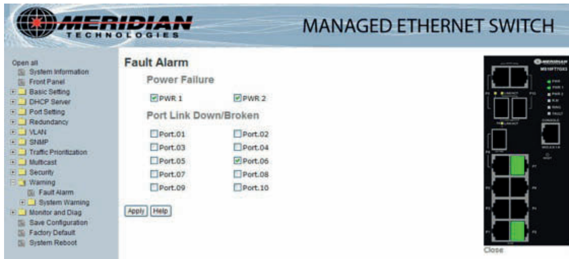
Fault Alarm interface
