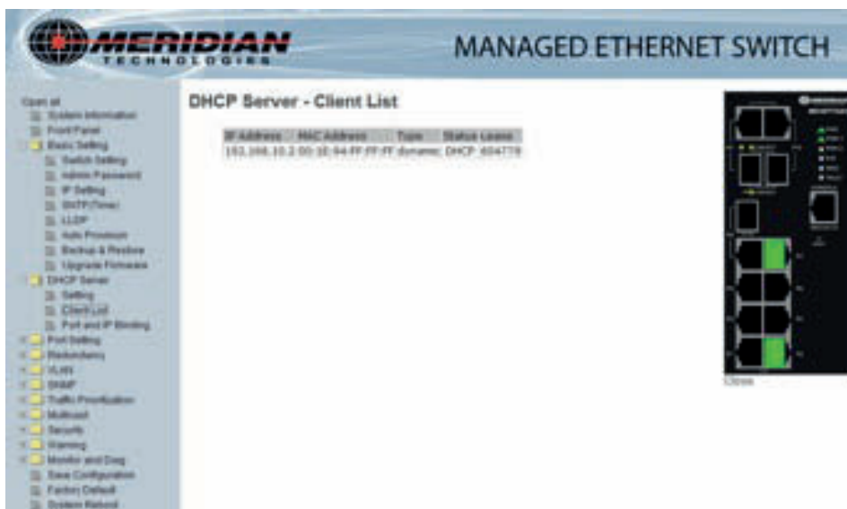
DHCP Server Client Entries interface
